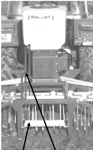
Steps and handrail
