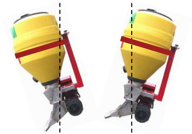
Additional frame is necessary, to avoid pulling out of hopper. Depending on the angle some seed can stay inside the hopper. The working width gets smaller the bigger the angle is.
